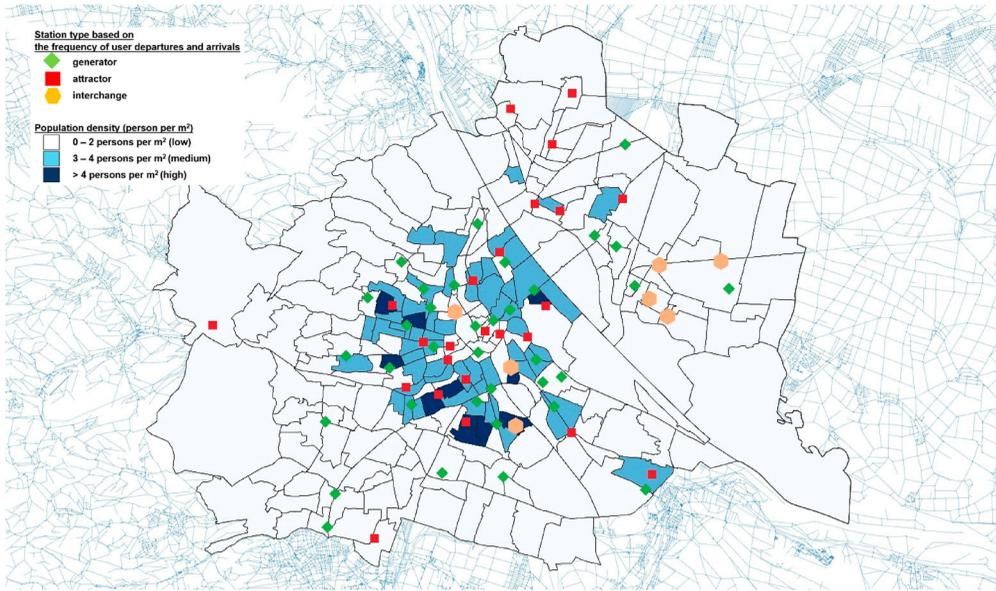
**Figure 14.** Optimal configuration of BS station with the station type.
