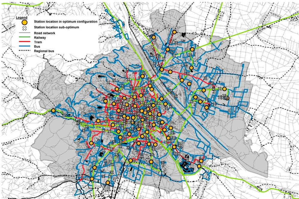
**Figure 15.** Optimal configuration of BS station with the transport network.
